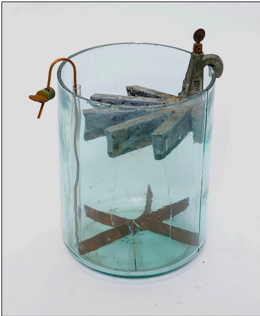
Figure 45. An early 20th-century (6" x 9.75") example of the crowfoot form of the Danzell gravity cell. The cast Zn crowfoot anode hangs from the edge of the jar and the star shaped Cu cathode rests on the bottom. Compare with figure 12.
