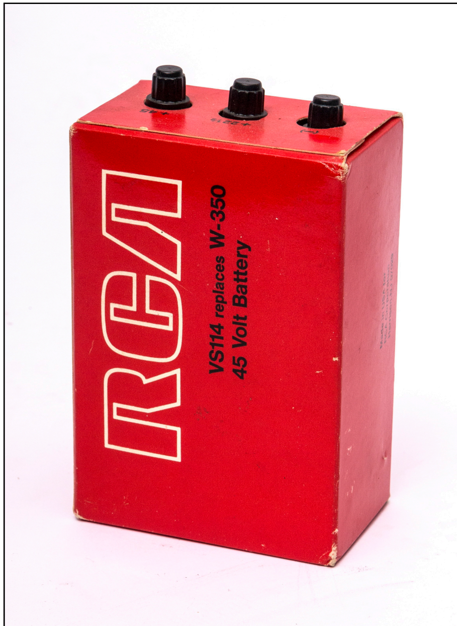
Figure 57. A circa 1960 (1.75" x 3" x 4.75") RCA 45 V battery pack composed of thirty small 1.5 V Leclanché "flat" dry cells.
