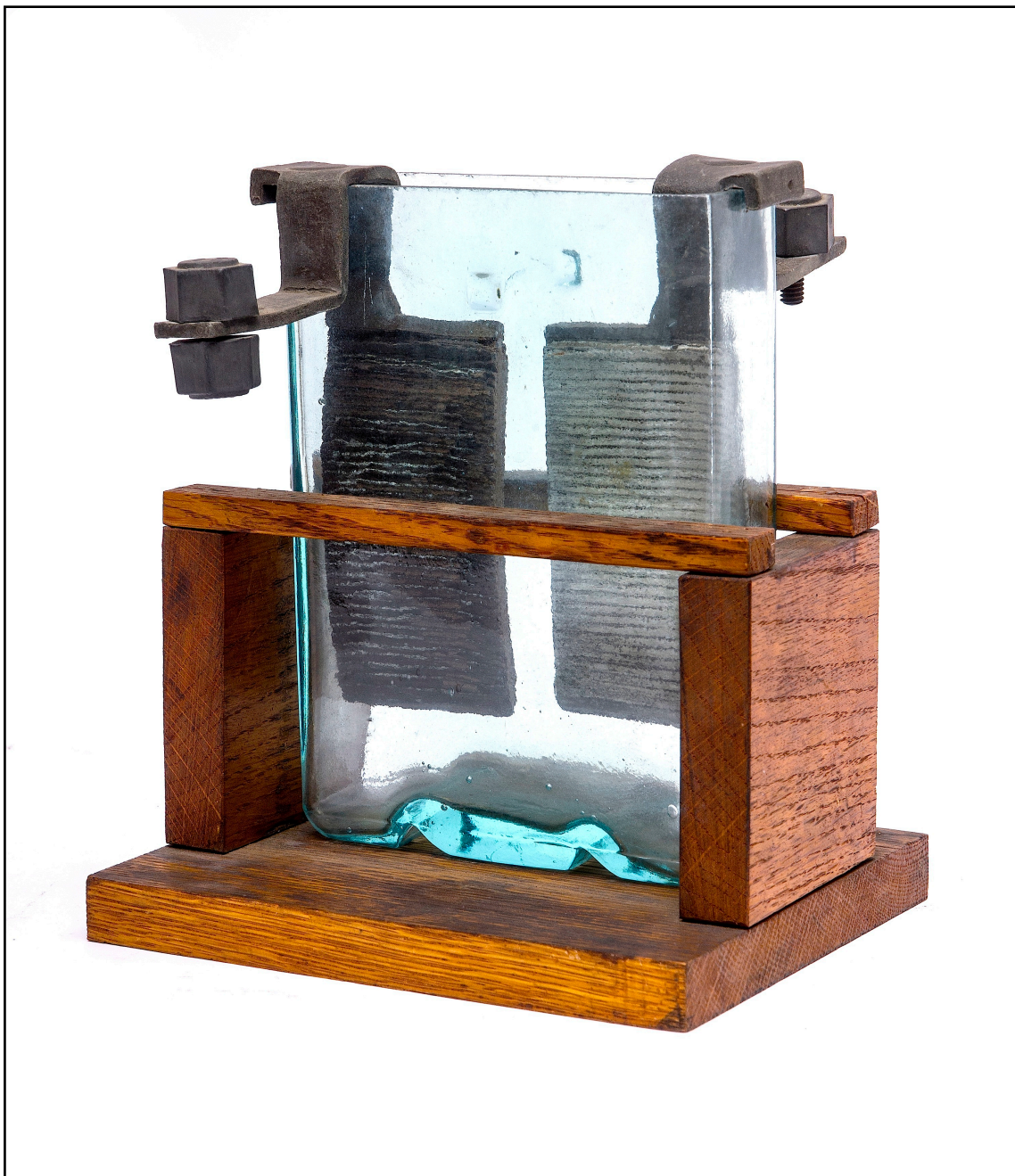
Figure 50. A circa 1920 handcrafted (5.75" x 6.75" x 7.5") Planté lead-acid cell with grooved electrodes made for use as a demonstration in the freshman chemistry course at Oberlin College.
