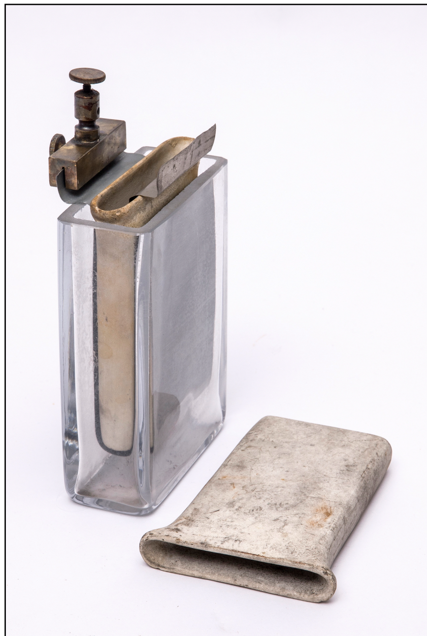
Figure 46. A 19th-century (2.5" x 3.5" x 7") example of a Grove nitric acid cell. The Zn anode is wrapped around the outside of the porous ceramic spacer and the Pt cathode is inside. A spare (0.5" x 3.25" x 4.5") ceramic spacer is shown on the right. Compare with figure 14.
