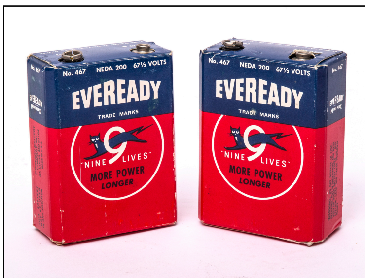
Figure 56. Two circa 1960 (1.25" x 2.75" x 3.5") 67.5 V EVEREADY battery packs each composed of forty-five small 1.5 V "flat" Leclanché dry cells.
