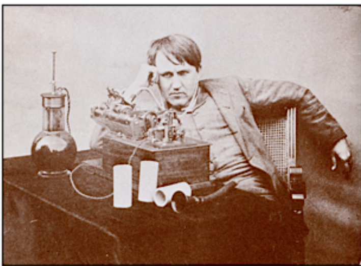
Figure 21. A famous photo of Thomas Edison posing in 1888 with his improved phonograph. Note the two-liter Grenet cell on the far left. Also note that its anode is in the raised position, thus indicating that it is not in operation.
