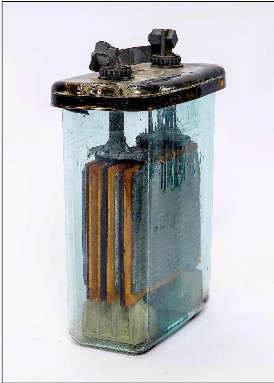
Figure 51. A circa 1960 (4.5" x 8" x 12.5") four cell lead storage battery that is an obvious descendent of the 1889 cell shown in figure 24. The name "Hyray" is molded into the side of the glass container.
