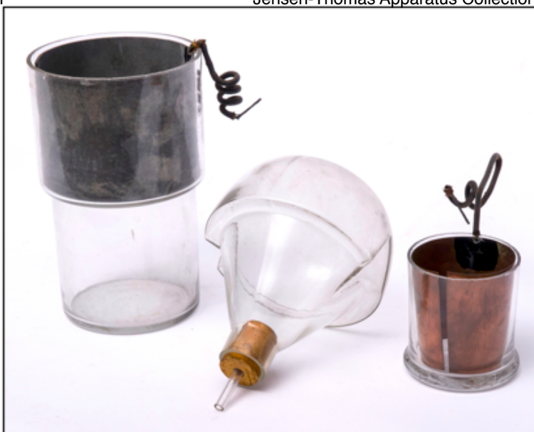
Figure 44. A disassembled Meidinger cell. From left to right: the outer cylinder and Zn anode, the globe or \text{Cu}(\text{SO}_4)(\text{s}) reservoir, and the inner cup and Cu cathode.
