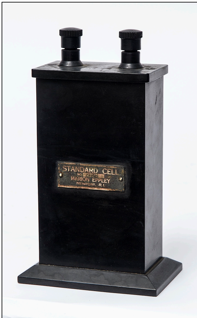
Figure 62. A circa 1920 (2.75" x 4.25" x 7.25") Weston cell in a Bakelite case made by the Eppley Laboratory of Newport RI. Compare with figure 38.
