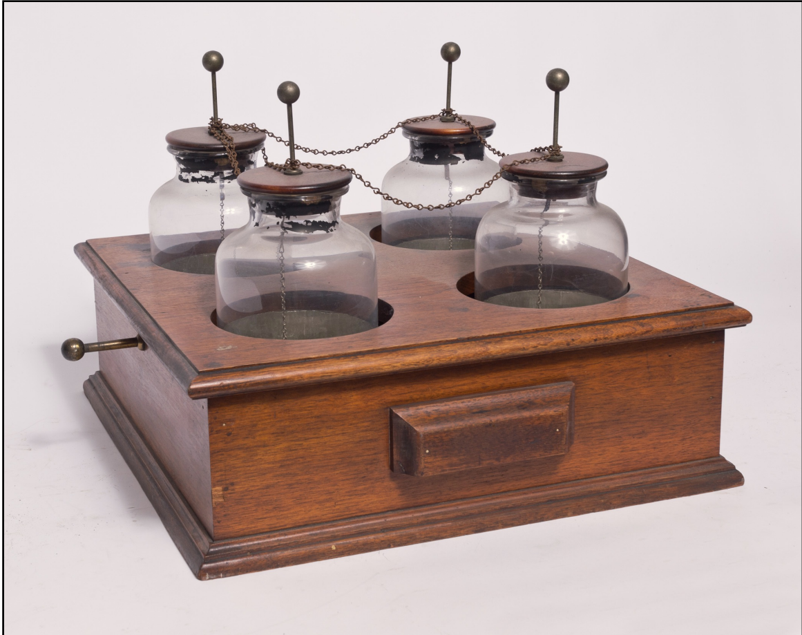
Figure 40. A 19th-century (13.5" x 20" x 20") "battery" of four interconnected half-gallon Leyden jars. Chains, rather than wires, were traditionally used to establish electrical contact.
