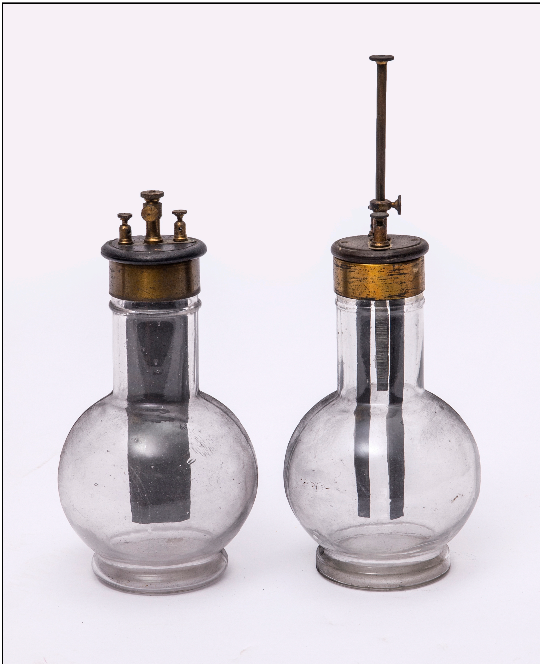
Figure 49. Two (4" x 8.25") 19th-century, half-liter Grenet dichromate cells. The Zn anode for the cell on the right is in the raised position. Compare with figure 20.
