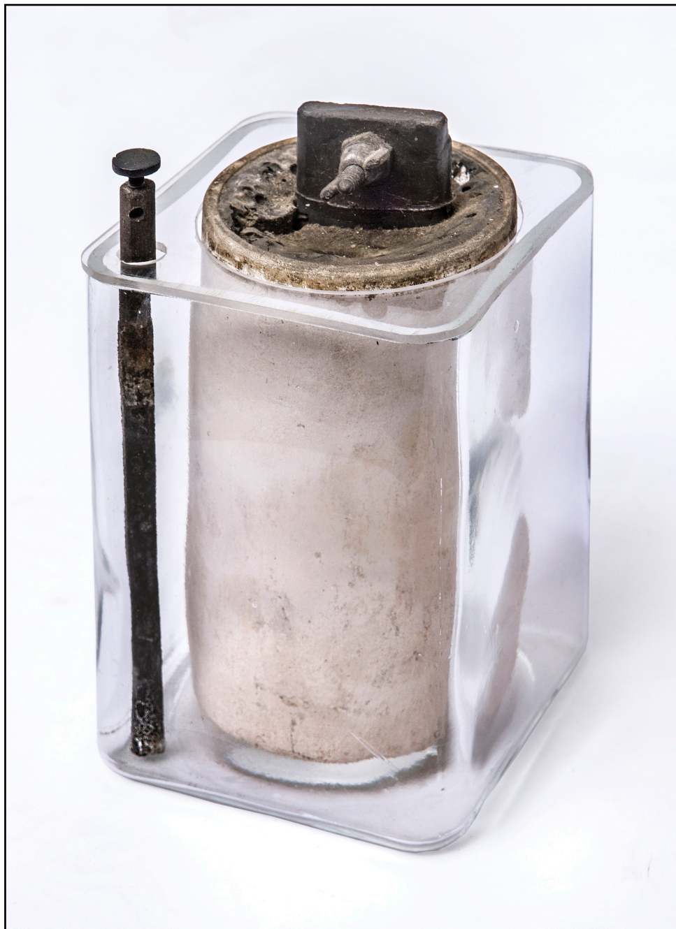
Figure 52. An early (4" x 4" x 7") wet Leclanché cell. The porous ceramic cylinder containing the graphite-MnO 2 mixture and the carbon block cathode is in the center and the Zn rod anode is on the far left. Compare with figure 27.
