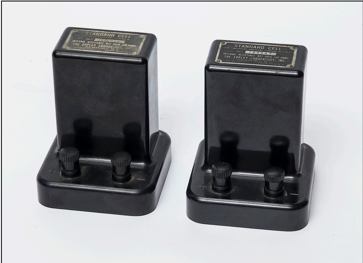
Figure 64. Circa 1940 precision grade (4" x 4" x 5") Weston cells in Bakelite cases made by the Eppley Laboratory of Newport RI.
