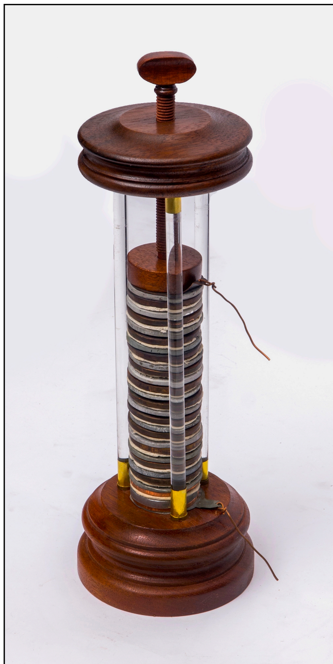
Figure 41. A modern (4.75" x 15") reproduction of a small voltaic pile. Compare with figure 6.
