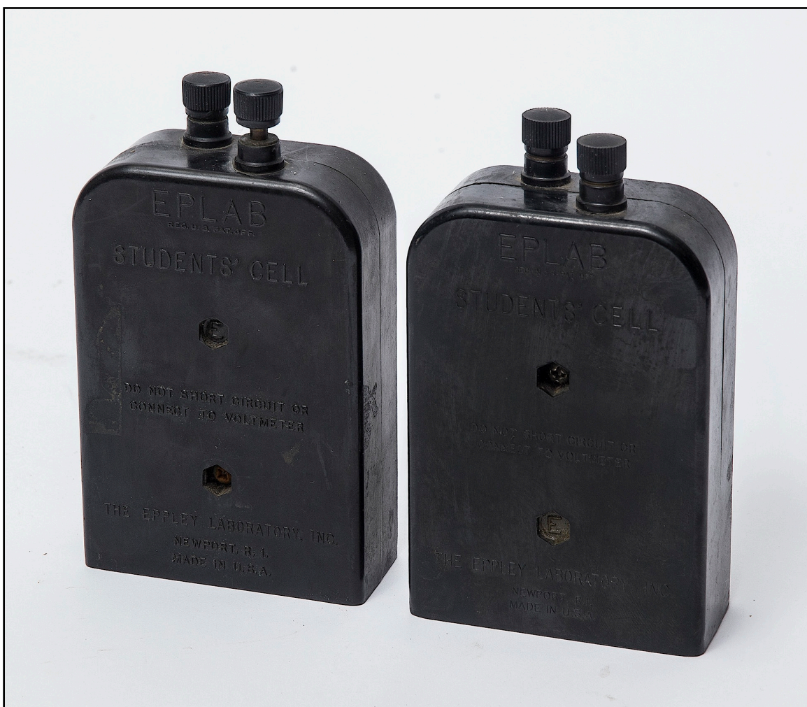
Figure 63. Circa 1940 “student” grade (1.25” x 3” x 5.25”) Weston cells in Bakelite cases made by the Eppley Laboratory of Newport RI.
