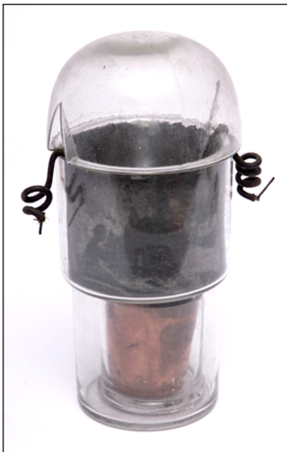
Figure 43. A late 19th-century (4" x 9") example of the globe or Meidinger form of the Daniell gravity cell. Compare with figure 11.
